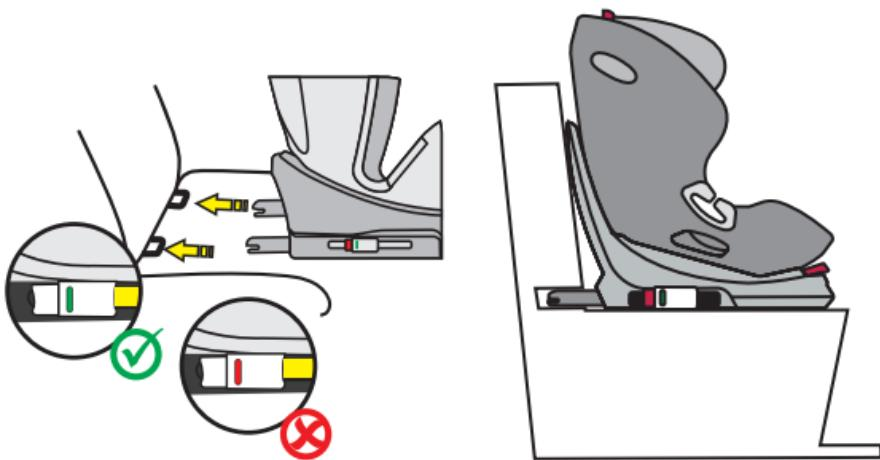
1. Press the two lateral Isofix connector buttons in order to extend the length of the Isofix connectors.
